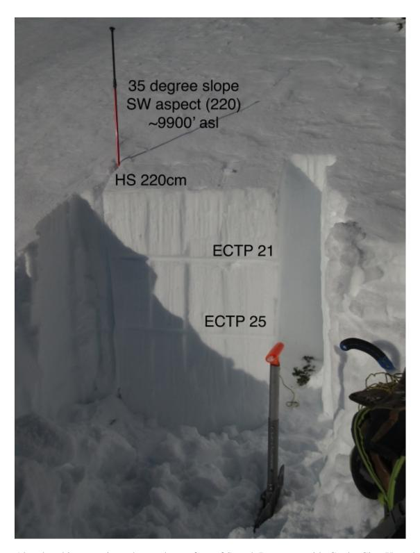
Alex dug this snowpit on the southwest face of Scotch Bonnet outside Cooke City. He only looked at the upper meter of snow and got propagation in his stability tests. Small facets on a crust were breaking and he did not ski the slope. Photo: GNFAC
